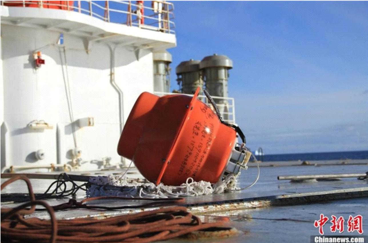
China's 28<sup>th</sup> Antarctic expedition team successfully recovered at 7:00 February 13<sup>th</sup>, 2012 two seabed seismometers (OBS) deployed two months ago at the Prydz Bay where the Chinese Zhongshan Station sits. A preliminary analysis of the recovered OBS indicates that the instruments worked smoothly on the ocean floor, with the data showing clear seismic signals.
